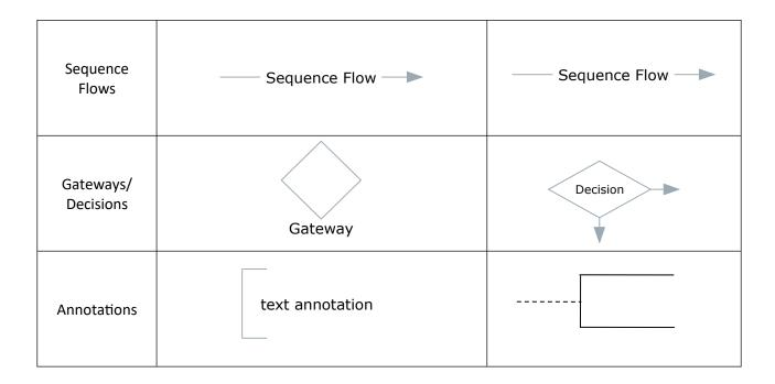
Comparing BPMN to data flow diagrams shows that the models are very different. Data flow diagrams do not have start, end, or intermediate event symbols. They do, however, clearly show the flow of data in a process or processes, where the BPMN diagram more clearly shows the sequence of activities.
