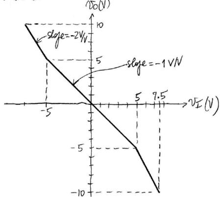
1.26 For NI > 0 we have No < 0, indicating that the opening ontput will prink current out of the inverting night mode. This mode is at victual ground, so D, will be off for NI > 0, and we only need to examine the following subcircuit:
