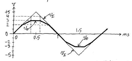
(b) Removing D2 and D4 will climinate the flat segments at the top and bottom; No will peak out at  $\pm (0.5 \times 5 + 1) = \pm 3.5 \text{ V}.$
