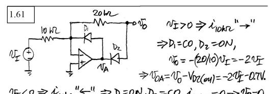
$V_{L}(0 \Rightarrow i_{10kn}" \leftarrow " \Rightarrow D_{1}=0N, D_{2}=co, i_{10kn}=0 \Rightarrow V_{0}=0.$   $V_{A}=V_{N}+V_{D1}(o_{1})=0+0.7=0.7V.$
