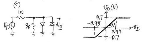
Now vo is clamped at ± 0.7V, and clamping occurs for  $|\nabla z| > \frac{1}{2} \times 0.7 = 0.93 \text{ V}$
