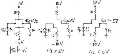
For  $|V_{\rm E}|$  2SV all diodes are on . April kCL to the diode supermode gives  $i + \frac{10-v_{\rm E}}{10} = \frac{v_{\rm E}}{10} + \frac{v_{\rm E}-(-10)}{10}$ , or  $i=0.3V_{\rm E}$ .
