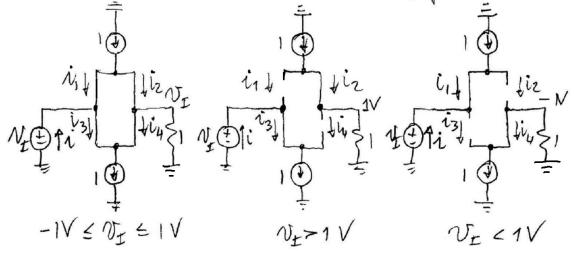
(a) For  $-1V \le V_{\pm} \le +1V$ , we apply kCL at the supermode,  $i+1=1+\frac{V_{\mp}}{I}$ , or  $i=V_{\pm}$ . Applying kCL further,  $i_1+i_2=1$ ,  $i_3+i_4=1$ ,  $i_3=i_1-i=i_1-V_{\pm}$ ;  $i_4=i_2-\frac{V_{\mp}}{I}=i_2-V_{\pm}$ . Combining,  $i_1+i_4=1-V_{\pm}$ , and  $i_2+i_3=1+V_{\pm}$ . But, by symmetry,  $i_1=i_4=(1-V_{\pm})/2$ , and  $i_2=i_3=(1+V_{\pm})/2$ . (b) For  $V_{\pm}>1V$ , i=1,  $i_1=i_4=0$ ,  $i_2=i_3=1$ .
