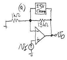
When diodes are off, we have  $N_0=(1+\frac{13}{4})VI=14$  VI. Clamping occurs for  $|V_0-V_M|=|V_0-V_L|=V_Z+2V_0(m)$ =5.1+1.4=6.5 V. This occurs
