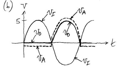
1.60 (a)  $N_N = U_P = 2.5V$ ;  $U_E > 2.5V \Rightarrow D_1 = 0N$ ,  $D_2 = 0KF$ ;  $N_0 = 2.5V$ ,  $N_A = 2.5 - 0.7 = 1.8V$ .  $N_E < 2.5V \Rightarrow D_1 = 0FF$ ,  $D_2 = 0N$ ,  $N_0 = V_N + R_2 I_{R2}$   $= N_N + R_2 I_{R_1} = N_N + R_2 (N_N - V_E)/R_1 = 5 - N_F$ .  $N_A = V_0 + 0.7$   $N_0(V)$
