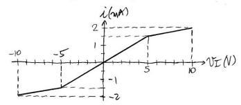
(b) As long as |VI|L5V, Ry has no effect as it is shorted out by the stronder, so i=0.3VI. For |VI|>5V, the source NI sees a resistance Reg = 10/[5+(10/10)]=5hr, so the slope of i vursus NI is now 1/kg =1/5=0.2mA/V. At the extremes, we have i = ±(1.5+0.2x5) = ±2.5 mA.
