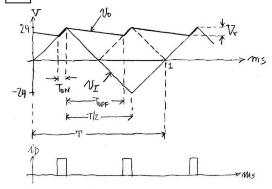
$V_0 = 24 - 2 \times 0.75 - \frac{1}{2} = 22 \text{ V}; I_0 = 22/2 = 11 \text{ mA}.$   $CV_4 = I_0 T_{0FF} = I_0 T/2 = I_0/(2f) \Rightarrow C = 11 \times 10^3/(2 \times 10^3 \times 1) = 5.5 \text{ mF}. ToN = (1/24)(1/4) = (1/24)(10^3/4) = 10.4 \text{ ms}$   $i_0(evg) = i_0(mac) = C \frac{V_4}{T_{0N}} + I_0 = (5.5 \times 10^6) \frac{1}{10.4 \times 10^6} + 11 \times 10^{-3}$  = 540 mA. PIV = 24V (make 35V to be Sofe).
