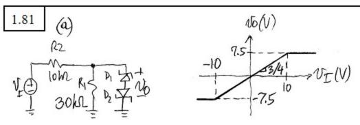
As long as both divides are off,  $V_0 = (3/4)VI$ . When biodes so on, they clamp  $V_0$  at  $\pm (V_2 + V_0) = \pm (6.8 + 0.7)$  =  $\pm 7.5 V$ . Clamping occurs for  $|V_I| > \frac{4}{3} \times 7.5 = 10 V$ .
