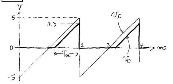
Of the diorde were ideal, we'd have Tow = T/z=1 ms (50% of T) and  $V_0(av_8) = \frac{(1\times5)/2}{2} = 1.75 \text{ V}$ . The error is therefore  $100 \frac{0.9245 - 1.75}{1.25} = -26\%$ .
