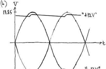
1.91 (a) let  $V_p = 2SV$ . Then,  $n = 25/(120 \times V_2) = 0.1493$ . Pick m = 0.15 (easier number). Then,  $V_p = 0.15 \times 120 V_2$  = 25.5V. let  $V_V = 2V$ . Then,  $V_{I}(min) = 25.5 - 0.8 - 2$ = 27.7 V.  $V_{Zo} = 15 - 0.01 \times 25 = 14.75V$ . Let  $I_{Z}(muin) = 5 \text{ mA}$ . Then,
