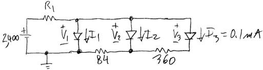
$$\begin{split} & I_3 = 0.1 \text{m} A = (1 \text{m} A)/10 \Rightarrow V_3 = 700 - 60 = 640 \text{m} V_0. \\ & V_2 = V_3 + R_3 I_3 = 540 + 360 \times 0.1 = 640 + 36 = 640 + 18 + 18 \\ & \Rightarrow I_2 = 0.1 \times 2 \times 2 = 0.4 \text{m} A. \\ & V_4 = V_2 + R_2 (I_2 + I_3) = 676 + 84(0.4 + 0.1) = 676 + 42 = \\ & I_18 = 700 + 18 \Rightarrow I_1 = 1 \times 2 = 2 \text{m} A. \\ & R_1 = (V_5 - V_1)/(I_1 + I_2 + I_3) = (2400 - 718)/(2 + 0.4 + 0.1) = 672.8 \ \Omega. \end{split}$$
