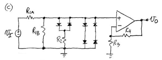
Impose RIA//RIB = 0.51 km, or FIA + RIB = 0.51, and I+RIA/RIB 5 = 2.2, or RIA/RIB = 1.27. Eliminating RIA, 1/(1.27 RIB) + 1/RIB = 1/0.51 => RIB = 0.91km, RIA=1.16 km. Firmelly, 5=(1+R4/R3)1.4 > R4/R3=2.57 > R3=20km, R4=51 km.
