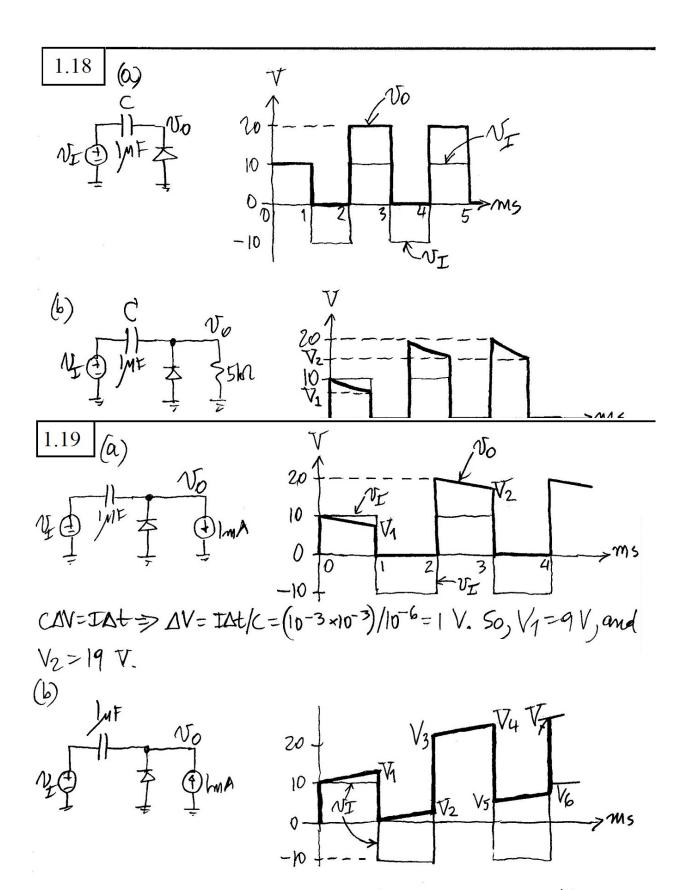
$V_1 = 10 + 1 = 11 \, \text{V}$ ,  $V_2 = 0 + 1 = 1 \, \text{V}$ ,  $V_3 = V_2 + 20 = 21 \, \text{V}$ ,  $V_4 = V_3 + 1 = 22 \, \text{V}$ ,  $V_5 = 22 - 10 = 2 \, \text{V}$ ;  $V_6 = V_5 + 1 = 3 \, \text{V}$ ,  $V_7 = V_6 + 20 = 23 \, \text{V}$ , and so on.
