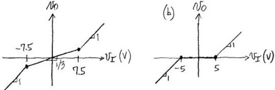
With the 20-br resistance removed, No=0 for (VE/SSV, No=NI-5 for NI >5, and No=NI+5 for NI <-5V.
