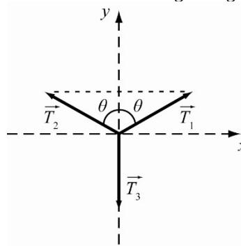
The horizontal components of  $T_1$  and  $T_2$  cancel out, so the sum  $T_1 + T_2$  is a vertical vector whose magnitude is  $T \cos \theta + T \cos \theta = 2T \cos \theta$ . The vector sum  $T_1 + T_2 + T_3$  is zero if  $2T \cos \theta - T = 0$
