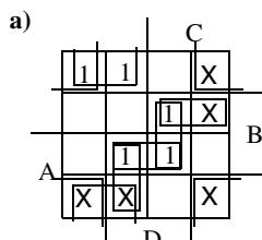
$$F = \bar{B}\bar{C} + BCD + ABD \quad F = X\bar{Y} + W\bar{Y}Z + WXZ + (\bar{W}\bar{X}Y \text{ or } \bar{W}Y\bar{Z}) \quad F = \bar{A} + \bar{C}$$
