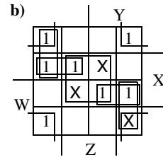
$$\text{Primes} = \bar{X}\bar{Z}, XZ, \bar{W}X\bar{Y}, WXY, \bar{W}Y\bar{Z}, WY\bar{Z}$$
