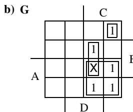
$$F = AC + \bar{A}\bar{B}\bar{C}D + \bar{A}\bar{B}\bar{C}\bar{D}$$
