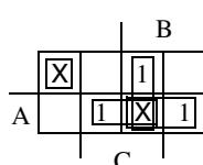
$$\text{Primes} = AB, AC, BC, \bar{A}\bar{B}\bar{C}$$
