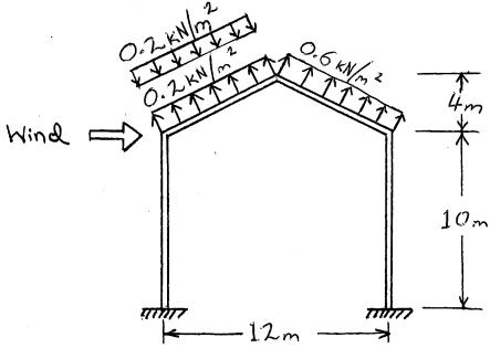
[2.11] V = 40m/s, E = 1.15, 3g = 274.32m,  $\alpha = 9.5$ From the solution of Problem 2.10:  $9h = 1.17 \, \text{kN/m}^2$  and G = 0.85
