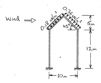
2.9 V=40 m/3, h=12+5=14.5m I=1.15, 8==366m, X=7.0, Kgt=1 and Ka = 1 K = 2.01 (14.5) = 0.8 J = 0.613(0.8)(1)(1)(40}(1.15) = 905-34 M/ms G=0.85 Roof 310pe: 0 = tan' (5/6) = 39.80  $\frac{h}{1} = \frac{14.5}{10} = 1.21$ CD = -0.1 and 0.25 for windward side Cp = -0.6 for leeward side Thus, the wind pressures are:
